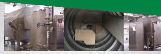
The IFT Series of drum thickeners offers best-in-class performance for sludge wastewater treatment. This sludge dewatering equipment is designed for achieving 5 to 12% solids depending on the type of sludge. The unit can handle solids loading up to 1900 lbs/hr (862 kg/hr) of WAS and 2850 lbs/hr (1293 kg/hr) for primary sludge, depending on the amount of solids content. The Monster Drum Thickener is designed to minimize operating costs while provide superior overall results.
